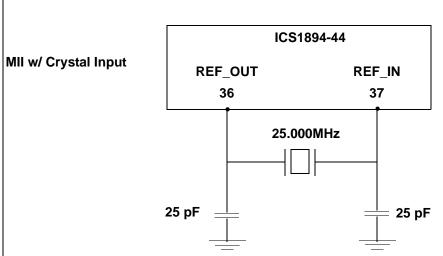
**NOTE:** 25 pF crystal load capacitors were required to bring the ppm for the 25 MHz crystal within the ±50 ppm on the IDT 1894 PHY evaluation board. The crystal used had a recommended load capacitance of 18 pF.
