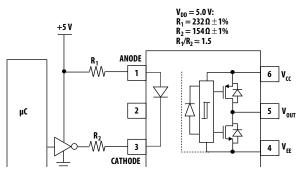
Figure 15 Recommended High-CMR Drive Circuit
