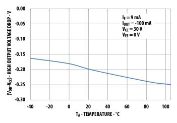
Figure 2 V<sub>OL</sub> vs. Temperature
