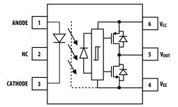
Note: A 1  $\mu F$  bypass capacitor must be connected between pins  $V_{CC}$  and  $V_{EE}.$
