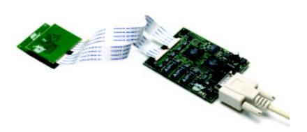
The AVR® ICE 200 In-Circuit Emulator is the perfect choice! A real-time In-Circuit Emulator based on a highly integrated AVR emulator chip. The ICE 200 speeds up the co-development of software and hardware for the world's fastest growing microcontroller family, the AVR 8-bit RISC. The ICE 200 emulator interfaces with AVR Studio®, Atmel's Integrated Development Environment (IDE) for code writing and debugging.
