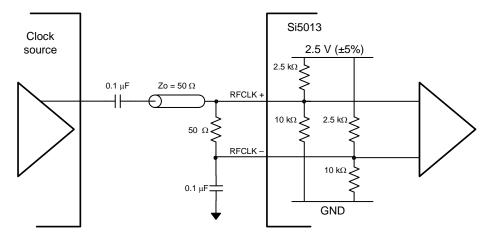
Figure 12. Single-Ended Input Termination for REFCLK (ac coupled)
