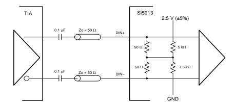
Figure 11. Input Termination for DIN (ac coupled)
