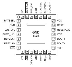
Figure 15. Si5013 Pin Configuration
