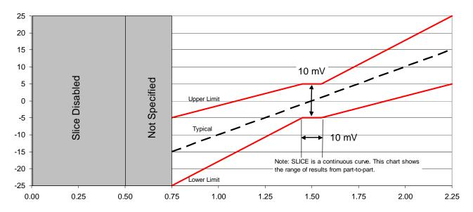
Figure 8. OC-12 and OC-3 Slice Specification
