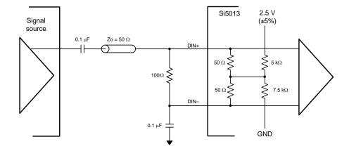
Figure 13. Single-Ended Input Termination for DIN (ac coupled)
