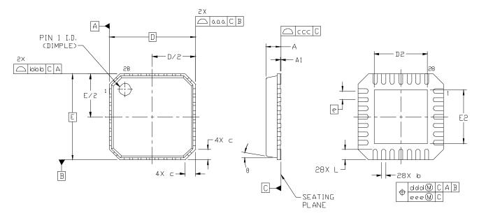
Figure 16. 28-Lead Quad Flat No-Lead (QFN)
