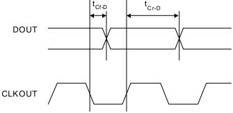
Figure 2. Clock to Data Timing
