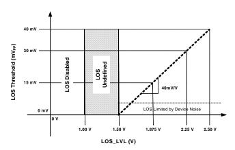
Figure 6. LOS\_LVL Mapping
