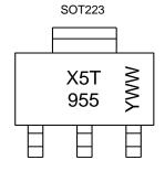
$\begin{array}{l} \text{X5T 955} = \text{Product Type Marking Code} \\ \text{YWW} = \text{Date Code Marking} \\ \text{Y or } \overline{\text{Y}} = \text{Last Digit of Year (ex: 5= 2015)} \\ \text{WW or } \overline{\text{WW}} = \text{Week Code (01~53)} \\ \end{array}$
