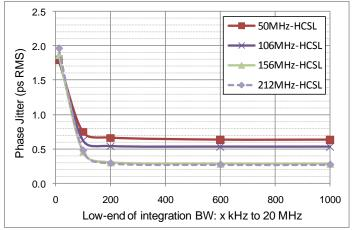
HCSL Phase jitter (integrated phase noise)
