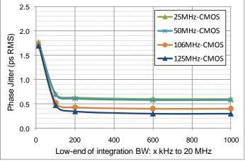
CMOS Phase jitter (integrated phase noise)
