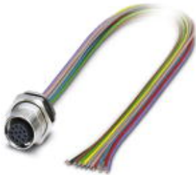
Sensor/actuator flush-type socket, 12-pos., M12 SPEEDCON, rear/screw mounting with Pg9 thread, with 0.5 m halogen-free TPE litz wire, 12 x 0.14 mm
