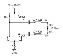
Figure 5c. CML AC-Coupled Termination (Vcco 1.8V only)
