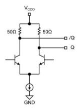
Figure 2b. Simplified CML Output Buffer
