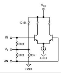
Figure 2a. Simplified Differential Input Buffer
