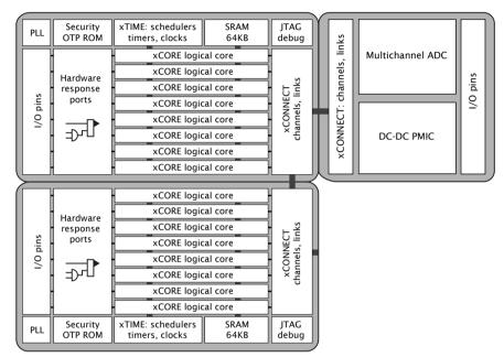
Figure 1: XS1-A Series:6-16 core devices
