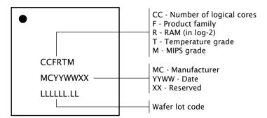
Figure 38: Part marking scheme
