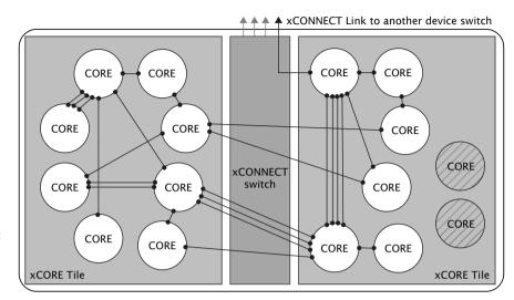
Figure 7: Switch, links and channel ends
