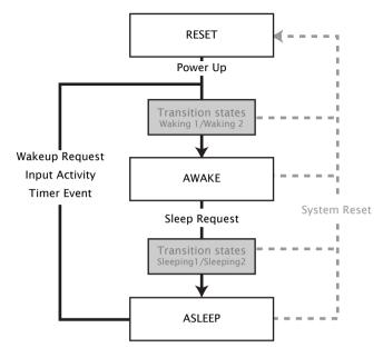
Figure 14: XS1-A8A-64-FB96 Power Up States and Transitions
