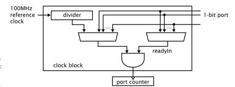
Figure 6: Clock block diagram
