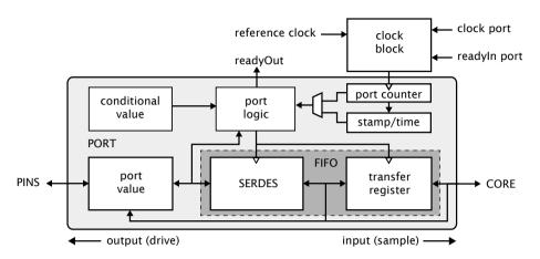
Figure 5: Port block diagram
