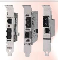
McPC Series Media Converters are ideal for Fiber-to-the-Desktop (FTTD) applications and for companies with frequent workstation moves and changes. Installing inside a PC or workstation, and plugging into an adjacent network interface card (NIC), these compact units eliminate the need to place Media Converters on top of desks or computers, reducing clutter of cords and adapters at the workspace.
