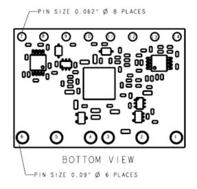
4.5 Vdc - 14 Vdc Input, 0.7 Vdc - 2 Vdc /50 A Outputs
