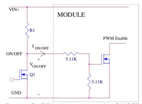
Remote On/Off Implementation using ON/OFF
