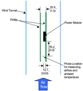
Thermal Test Setup
