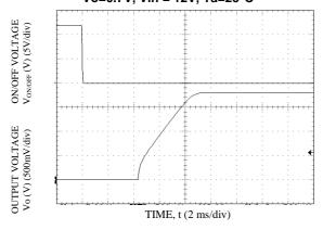
Start-up Using On/Off Voltage (Io = Io,max) Vo=1.8V, Vin = 12V, Ta=25°C
