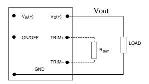
Circuit configuration to program output voltage using an external resistor
