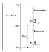
Circuit Configuration for margining Output voltage
