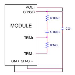
Circuit diagram showing connection of  $R_{\text{TUNE}}$  and  $C_{\text{TUNE}}$  to tune the control loop of the module
