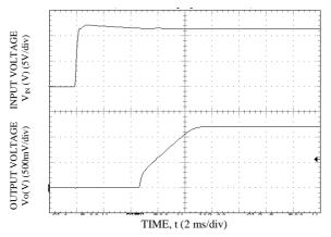
Start-up Using Input Voltage ( $V_{IN} = 12V$ ,  $I_o = I_{o,max}$ ),  $V_o=1.2V$ ,  $T_a=25$ °C
