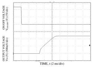
Start-up Using On/Off Voltage (Io = Io,max) Vo=1.2V, Vin = 12V, Ta=25°C
