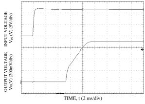
Start-up Using Input Voltage (V<sub>IN</sub> = 12V, Io =  $I_{o,max}$ ), Vo=0.7V, Ta=25°C
