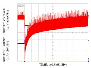
Transient Response to Dynamic Load Change from 50% to 100%. Vo=1.2V, Ta=25°C, Vin=12V, Cext =5x47uF+ +13x330uFpolymer,CTune=120nF,RTune=180ohms
