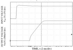
Start-up Using Input Voltage ( $V_{IN} = 12V$ ,  $I_0 = I_{o,max}$ ),  $V_0 = 1.8V$ ,  $T_0 = 12V$ ,  $I_0 = I_{o,max}$ ),
