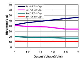
4.5 Vdc - 14 Vdc Input, 0.7 Vdc - 2 Vdc /50 A Outputs
