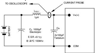
NOTE: Measure input reflected ripple current with a simulated source inductance ( $L_{\text{TEST}}$ ) of 1µH. Capacitor  $C_{\text{S}}$  offsets possible battery impedance. Measure current as shown above.
