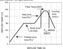
Reflow Profile for Tin/Lead (Sn/Pb) process
