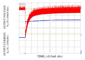
Transient Response to Dynamic Load Change from 50% to 100%. Vo=1.8V, Ta=25°C, Vin=12V, Cext =5x47uF+ +8x330uFpolymer,CTune=47nF,RTune=220ohms
