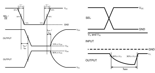
Figure 5. t<sub>EN</sub>, t<sub>DIS</sub>, t<sub>ON</sub>, t<sub>OFF</sub> Times
