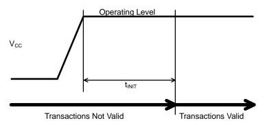
Figure 4.  $t_{INIT}$ , Initialization Time
