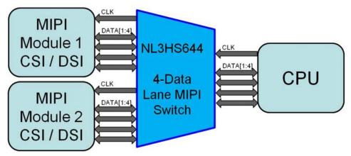
Figure 1. Typical Application - Mobile Phone
