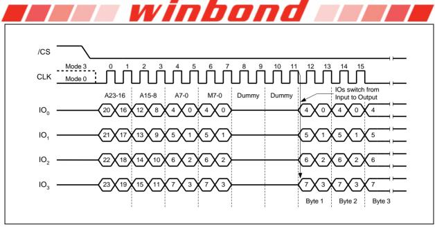
Figure 24b. Fast Read Quad I/O Instruction (Previous instruction set M5-4 = 10, SPI Mode) 32-Bit Address is required when the device is operating in 4-Byte Address Mode
