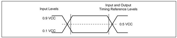
Figure 59. AC Measurement I/O Waveform
