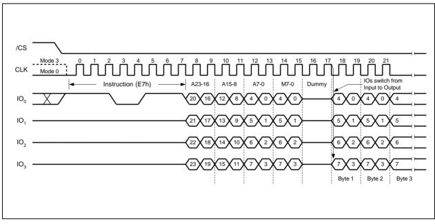
Figure 26a. Word Read Quad I/O Instruction (Initial instruction or previous M5-4  $\neq$  10, SPI Mode only) 32-Bit Address is required when the device is operating in 4-Byte Address Mode
