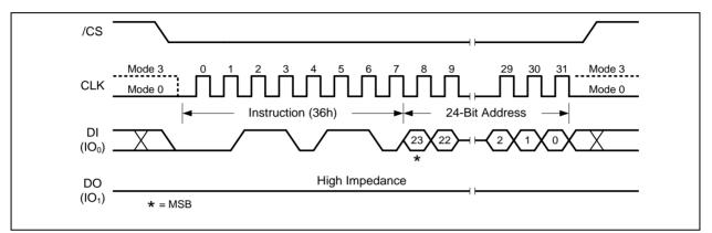
Figure 52a. Individual Block/Sector Lock Instruction (SPI Mode) 32-Bit Address is required when the device is operating in 4-Byte Address Mode
