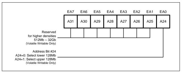
Figure 4e. Extended Address Register
