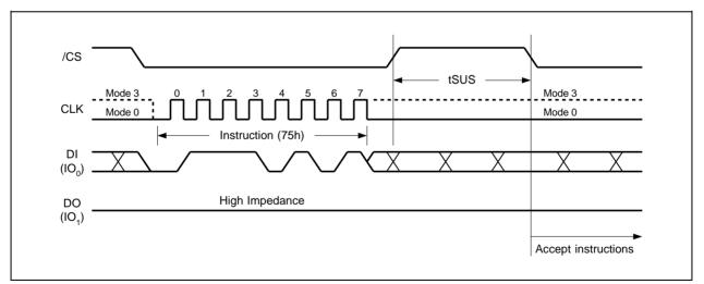
Figure 35a. Erase/Program Suspend Instruction (SPI Mode)
