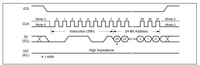
Figure 53a. Individual Block Unlock Instruction (SPI Mode) 32-Bit Address is required when the device is operating in 4-Byte Address Mode
