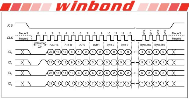
Figure 29b. Page Program Instruction (QPI Mode) 32-Bit Address is required when the device is operating in 4-Byte Address Mode
