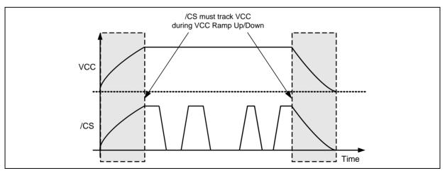
Figure 58b. Power-up, Power-Down Requirement
