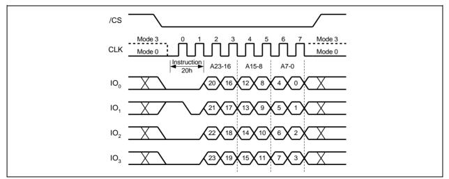
Figure 31b. Sector Erase Instruction (QPI Mode) 32-Bit Address is required when the device is operating in 4-Byte Address Mode
