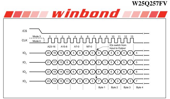
Figure 27b. Octal Word Read Quad I/O Instruction (Previous instruction set M5-4 = 10, SPI Mode only) 32-Bit Address is required when the device is operating in 4-Byte Address Mode
