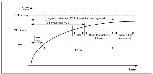
Figure 58. Power-up Timing and Voltage Levels
