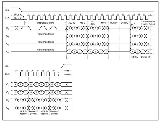
Figure 41. Read Manufacturer / Device ID Quad I/O Instruction (SPI Mode only) 32-Bit Address is required when the device is operating in 4-Byte Address Mode
