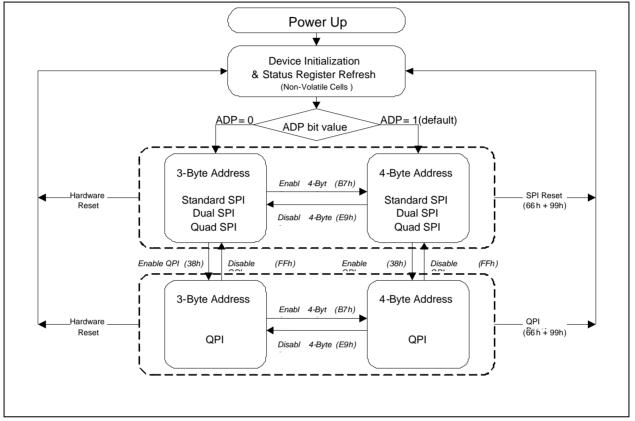
Figure 3. W25Q257FV Serial Flash Memory Operation Diagram
