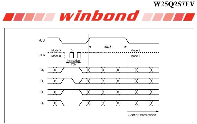
Figure 35b. Erase/Program Suspend Instruction (QPI Mode)
