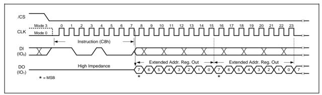
Figure 10a. Read Extended Address Register Instruction (SPI Mode)
