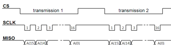
Figure 11: Timing Diagram for Simple SPI Readout
