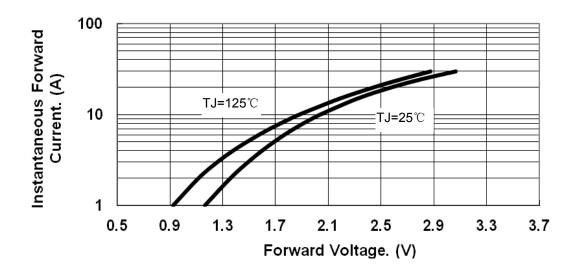
Fig.3-Typical Instantaneous Forward Voltage Characteristics
