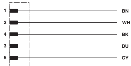
Contact assignment of the M12 plug
