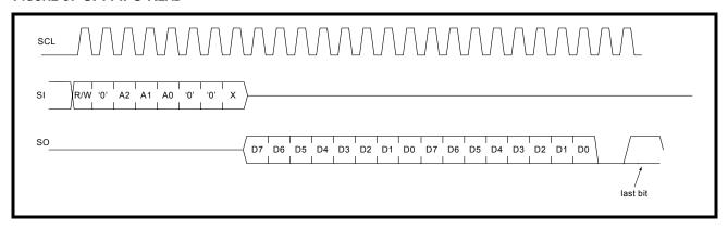
After the last read or write transaction, the SPI master will set the SCL signal back to its idle state (LOW).
