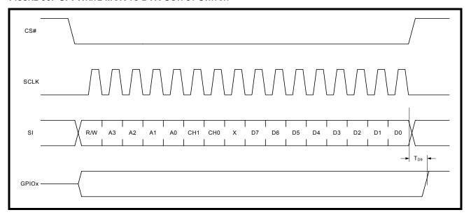
FIGURE 31. SPI WRITE MCR TO DTR OUTPUT SWITCH
