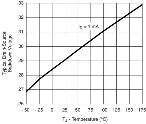
Typical Drain-Source Brakdown Voltage vs. Junction Temperature
