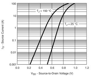
Source-Drain Diode Forward Voltage
