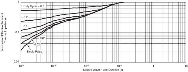
Normalized Thermal Transient Impedance, Junction-to-Case
