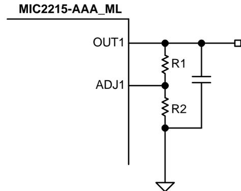
Figure 1. Adjustable Output
