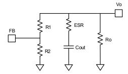
Figure 8—Simplified Circuit in skip Mode
