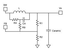
Figure11—Simplified Circuit of Ceramic Capacitor
