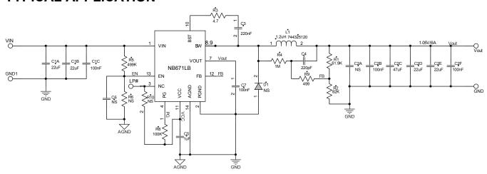
Figure 14 — Typical Application Circuit For NB671LB  $V_{IN}$ =4.5-22V,  $V_{OUT}$ =1.05V,  $I_{OUT}$ =6A
