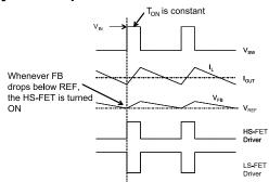
Figure 2—Heavy Load Operation
