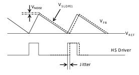
Figure 4—Jitter in PWM Mode
