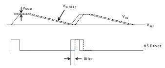
Figure 5—Jitter in Skip Mode
