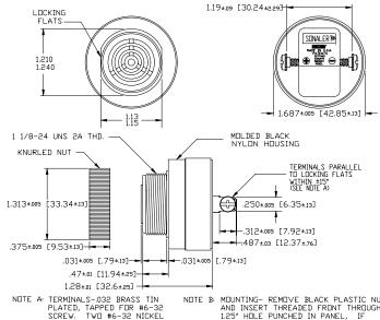
NOTE A: TERMINALS-032 BRASS TIN PLATED, TAPPED FOR #6-32 SCREW. TWO #6-32 NICKEL PLATED BRASS SCREWS INCLUDED. WILL ACCEPT 1/4\* QUICK CONNECT.
