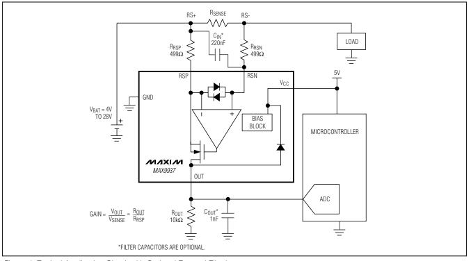
Figure 1. Typical Application Circuit with Optional External Filtering
