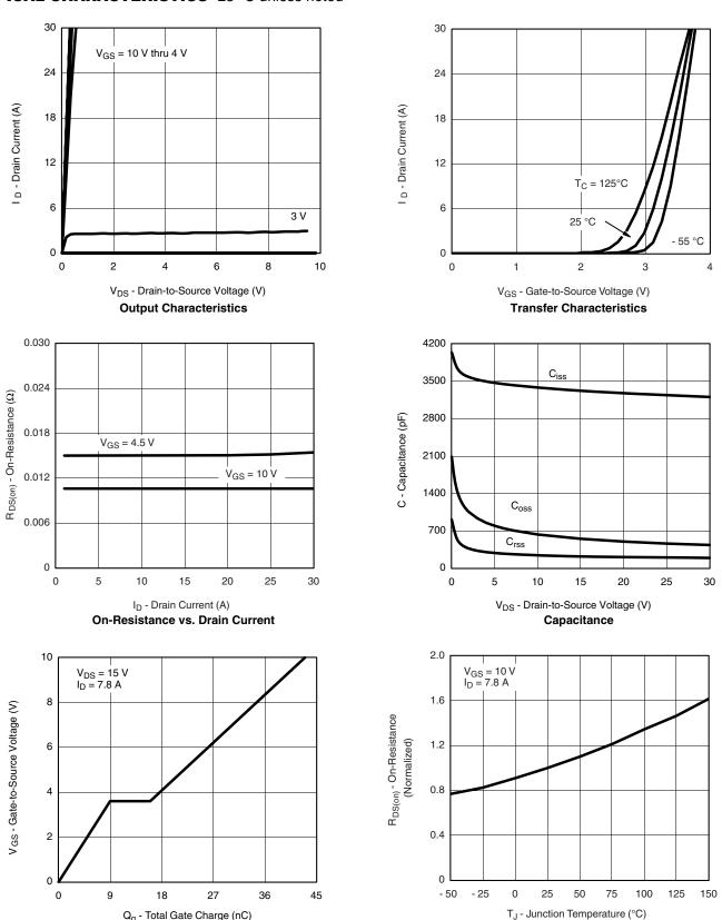
$Q_g$  - Total Gate Charge (nC) **Gate Charge**
