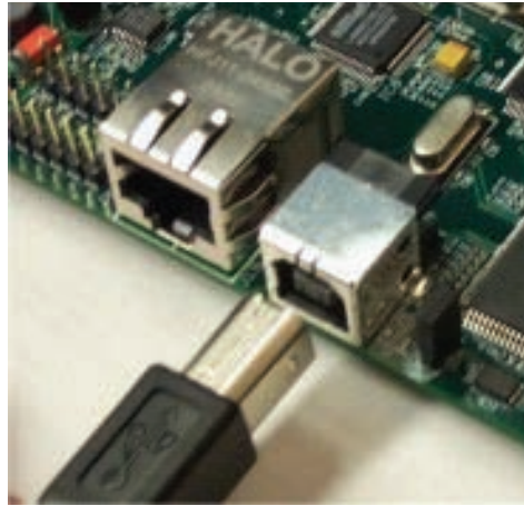
Figure 4-3: Connect the USB Type B Connector to the Starter Kit Board Connector
