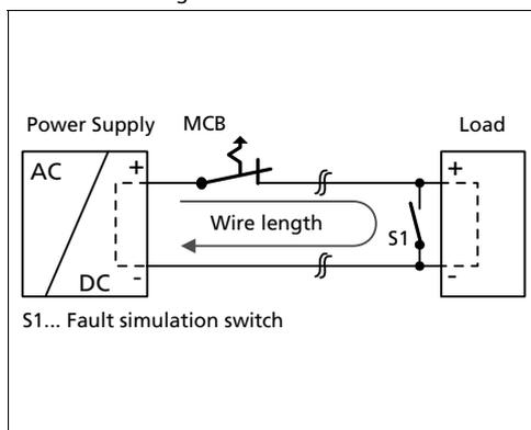
Maximal wire length\*) for a fast (magnetic) tripping:
