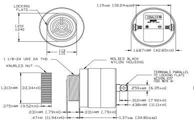
NOTE A: TERMINALS-.032 BRASS TIN PLATED, TAPPED FOR #6-32 SCREW. TVOI #6-32 NICKEL PLATED BRASS SCREWS INCLUDED. WILL ACCEPT 1/4' QUICK CONNECT.
