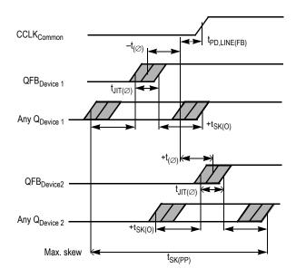
Figure 8. MPC9773 Maximum Device-to-Device Skew
