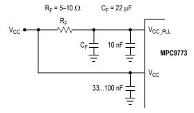
Figure 7. V<sub>CC\_PLL</sub> Power Supply Filter
