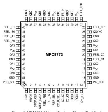
Figure 2. MPC9773 52-Lead Package Pinout (Top View)
