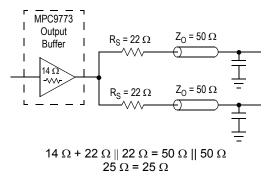
Figure 14. Optimized Dual Line Termination
