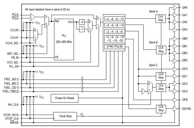
Figure 1. MPC9773 Logic Diagram
