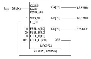
MPC9773 example configuration (feedback of QFB = 25 MHz,  $f_{VCO}$  = 250 MHz,  $VCO\_SEL$  =  $\div$ 1, M = 10,  $N_A$  = 4,  $N_B$  = 4,  $N_C$  = 2).
