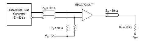
Figure 16. PCLK MPC9773 AC Test Reference
