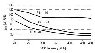
Figure 11. MPC9773 I/O Jitter
