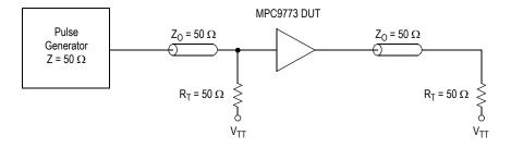
Figure 15. CCLK MPC9773 AC Test Reference
