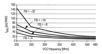
Figure 9. MPC9773 I/O Jitter
