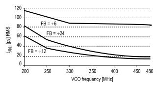
Figure 10. MPC9773 I/O Jitter
