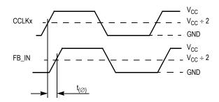
Figure 18. Propagation Delay  $(\mathbf{t}_{(\varnothing)},$  Static Phase Offset) Test Reference
