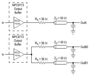
Figure 12. Single versus Dual Transmission Lines
