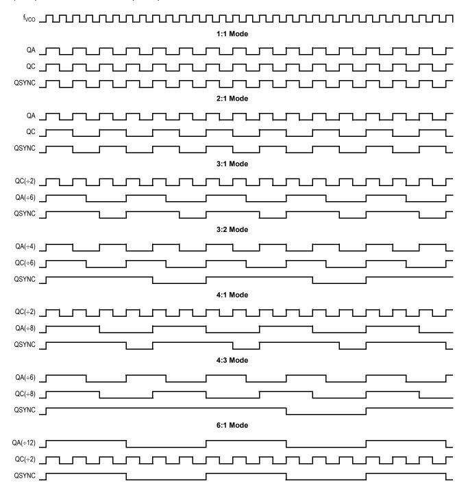
Figure 6. QSYNC Timing Diagram
