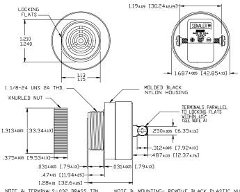
NOTE A: TERMINALS-032 BRASS TIN PLATED, TAPPED FOR #6-32 SCREW, TWD #6-32 NICKEL PLATED BRASS SCREWS INCLUBED, WILL ACCEPT 1/4\* QUICK CONNECT. NOTE B: MOUNTING- REMOVE BLACK PLASTIC NUT AND INSERT THREADED FRONT THROUGH 1.25' HOLE PUNCHED IN PANEL, IF DRIENTATION IS NEEDED, NOTE LOCKING FLATS ON DRAVING, SCREW NUT BACK ON. DO NOT DVERTIGHTEN.
