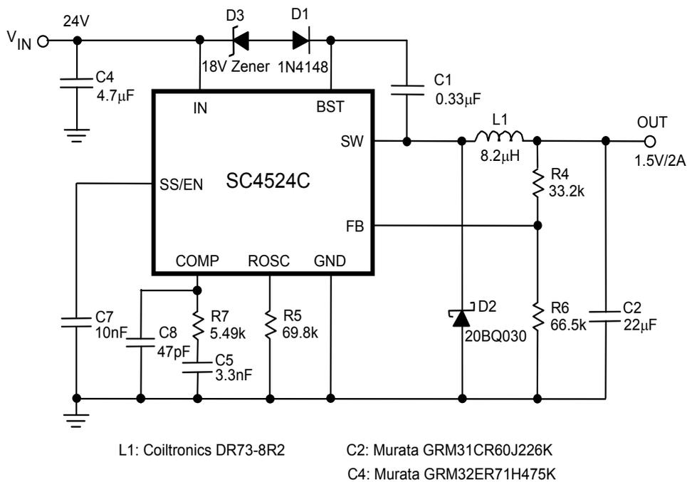
**Figure 10. 300kHz 24V to 1.5V/2A Step-down Converter**
