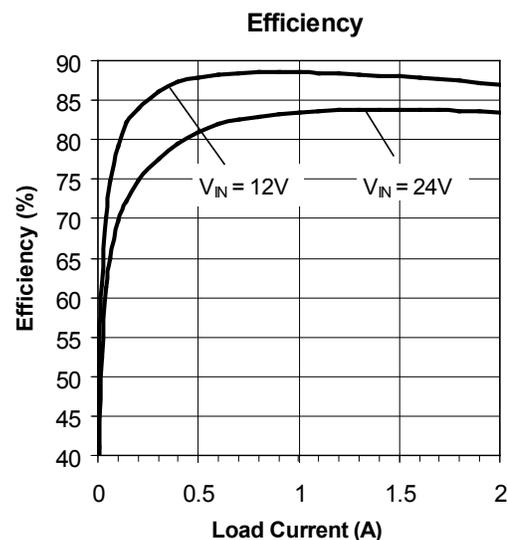
Figure 1. 1MHz 10V-28V to 5V/2A Step-down Converter
