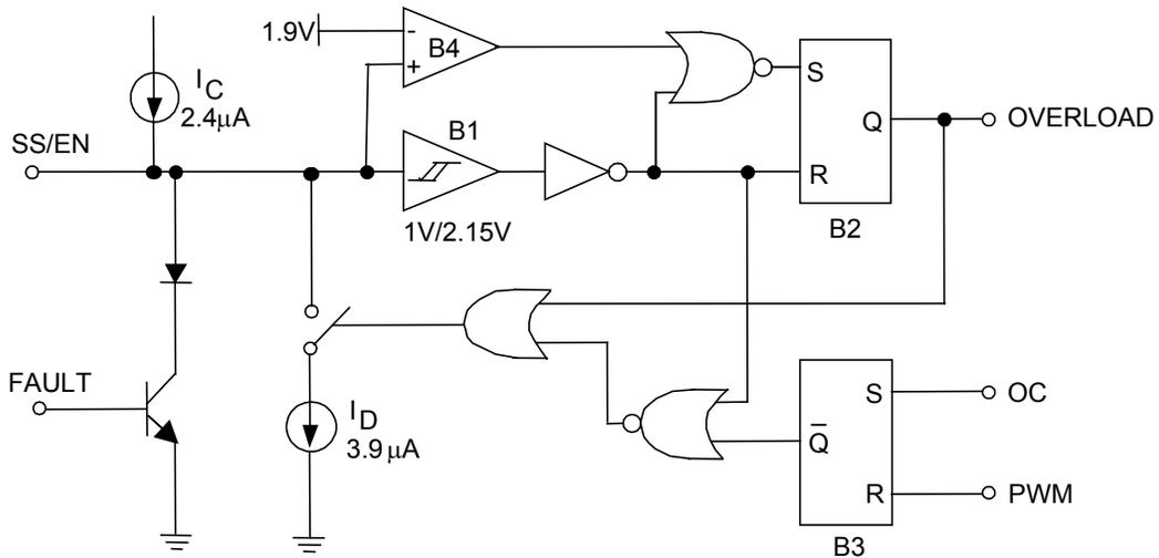
Figure 3 — Soft-start and Overload Hiccup Control Circuit
