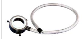
Fiber Optic Ring Light, with its continuous ring, is the most popular light transmitter. The ring light housing encases high-quality glass fibers to provide 360° shadow-free uniform illumination that makes viewing of inspection and assembly applications a snap. Its 36" cable, made with interlocking stainless steel sheathing, enables the illuminator to be positioned outside the immediate work area to provide more space for inspection and assembly operations.
