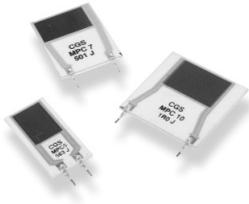
A range of non inductive thick film power resistors complementing the T0220 packaged MPR series (20 Watt heat sink styles), being vertically mounted and suitable to dissipate power from 3 Watts up to 10 Watts. Available in values from 1R0 to 200K ohms they are the idea solution for small snubber circuits, the output side of high speed pulse generators and low inductive resistor requirements in switch mode power supplies.
