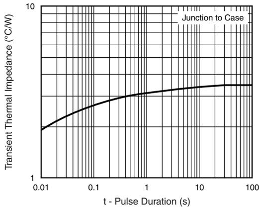
Fig. 5 - Typical Transient Thermal Impedance Per Diode
