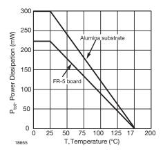
Fig. 1 - Steady State Power Derating Curve
