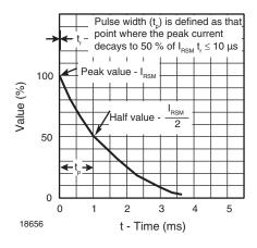
Fig. 2 - Pulse Waveform
