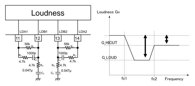
Figure 17. About the External Parts Setting of Loudness Circuit
