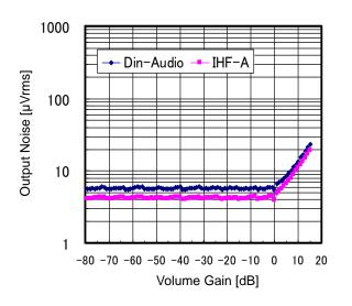
Figure 7. Output Noise vs Volume Gain
