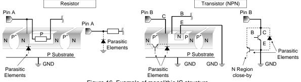
Figure 16. Example of monolithic IC structure
