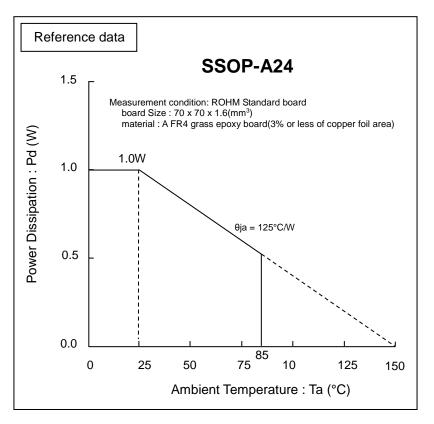
Figure 15. Temperature Derating Curve
