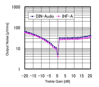
Figure 9. Output Noise vs Treble Gain
