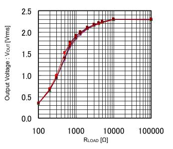
Figure 10. Output Voltage vs RLOAD
