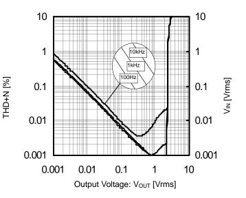
Figure 2. THD+N vs Output Voltage
