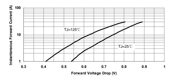
Fig.3-Typical Instantaneous Forward Voltage Characteristics
