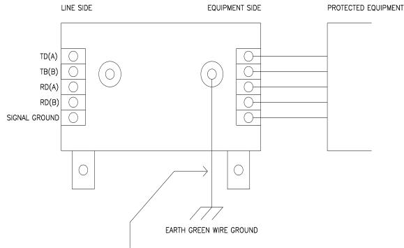
10 GAUGE COPPER WIRE AT 3 FEET LONG. OR BRAIDED CABLE MADE SPECIFICALLY FOR GROUNDING PURPOSES.
