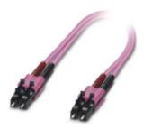
Assembled FO cable, zip cord cable, multi-mode fiberglass 50/125 µm, OM4, plug: LC/LC, degree of protection: IP20, for installation in cable ducts or control cabinets, length: 1 m
