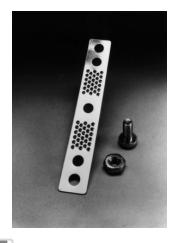
The 4464 shield bond connector is a strip of tin-plated brass, punched with mounting holes and two sets of sharp teeth. Each connector can join the shields of up to four two-pair service wires to a stud type shield connector.
