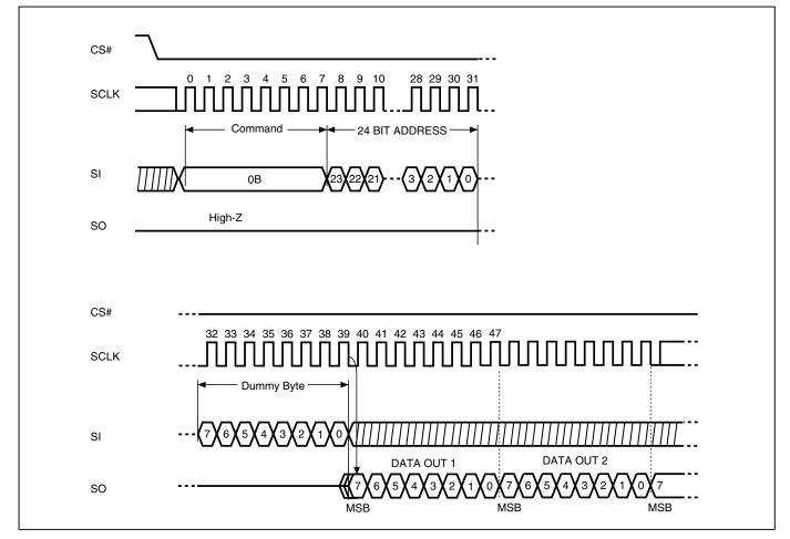
Figure 18. Dual Output Read Mode Sequence (Command 3B)
