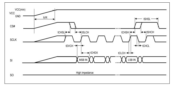
Figure 28. AC Timing at Device Power-Up
