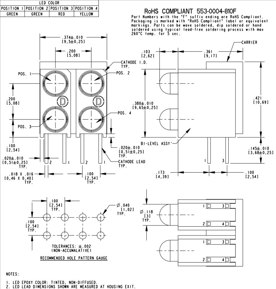
3. LEADS TO FIT INTO HOLES SPACED AS PER PATTERN.
