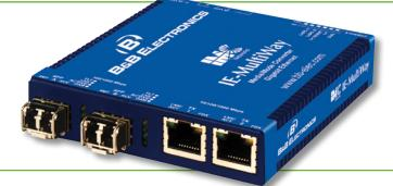
The IE-MultiWay is a value-based, Carrier-class managed Gigabit Ethernet solution that is ideal for use as a CPE device at the customer's network edge as well as in a fiber infrastructure. The IE-MultiWay comes standard with two SFP uplink ports for the providers' network connection and two 10/100/1000Base-T copper ports.
