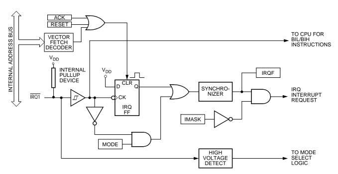
Figure 12-1. IRQ Module Block Diagram
