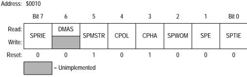
Figure 20-13. SPI Control Register (SPCR)
