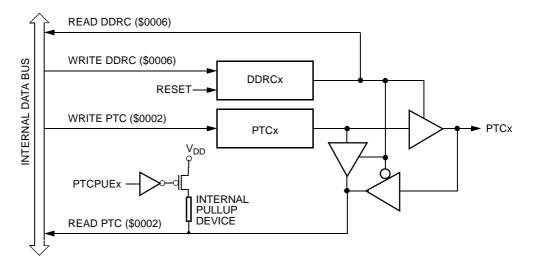
Figure 16-11. Port C I/O Circuit
