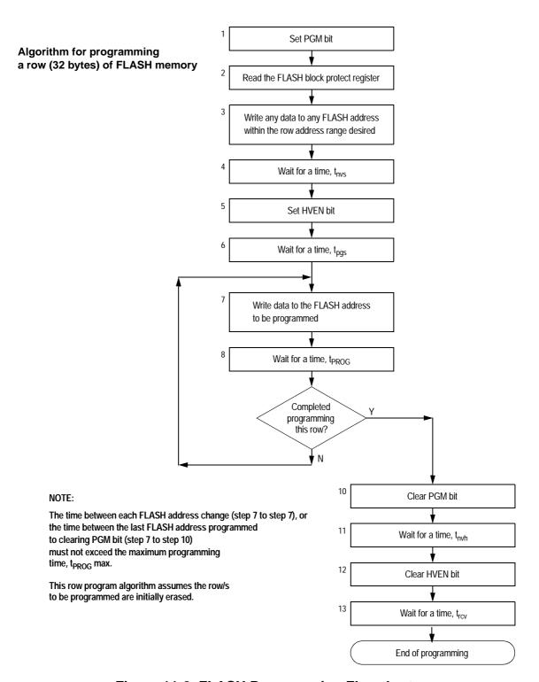
Figure 11-2. FLASH Programming Flowchart
