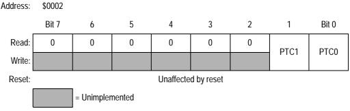
Figure 16-9. Port C Data Register (PTC)
