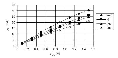
$V_{OL} < 0.4 \text{ V } @ I_{OL} = 1.6 \text{ mA}$  $V_{OL} < 1.5 \text{ V } @ I_{OL} = 10.0 \text{ mA}$
