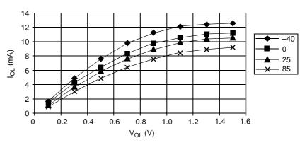
$V_{OL} < 0.3 \ V @ I_{OL} = 0.5 \ mA$  $V_{OL} < 1.0 \ V @ I_{OL} = 6.0 \ mA$
