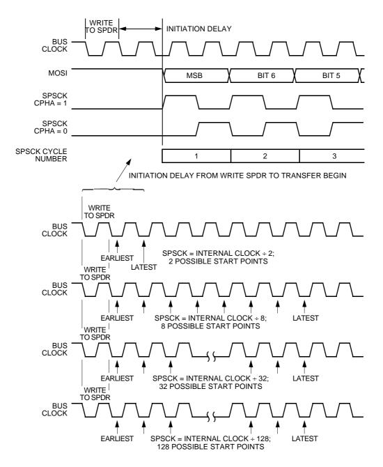
Figure 20-7. Transmission Start Delay (Master)
