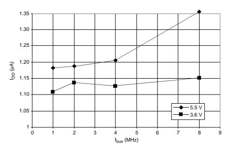
Figure 23-15. Typical Stop Mode  $I_{DD}$ , with all Modules Disabled (-40  $^{\circ}$ C to 125  $^{\circ}$ C)
