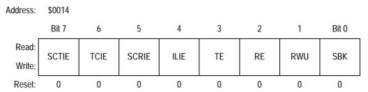
Figure 18-10. SCI Control Register 2 (SCC2)
