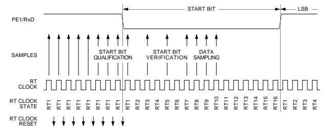
Figure 18-6. Receiver Data Sampling
