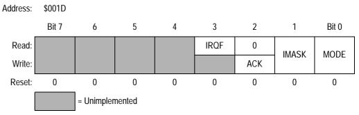
Figure 12-3. IRQ Status and Control Register (INTSCR)
