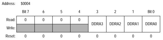
Figure 16-3. Data Direction Register A (DDRA)
