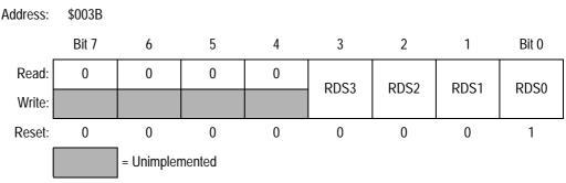
Figure 7-9. PLL Reference Divider Select Register (PMDS)
