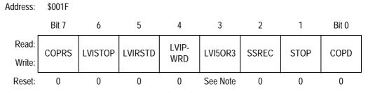
Note: LVI5OR3 bit is only reset via POR (power-on reset)
