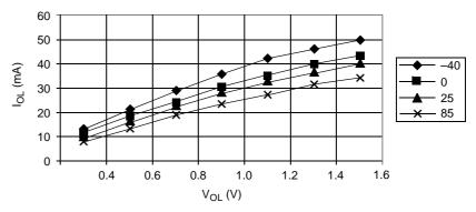
$V_{OL}$  < 1.0 V @  $I_{OL}$  = 15 mA
