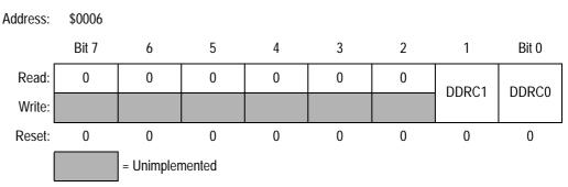
Figure 16-10. Data Direction Register C (DDRC)
