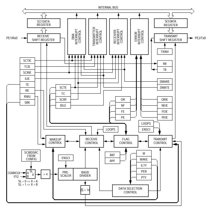
Figure 18-1. SCI Module Block Diagram
