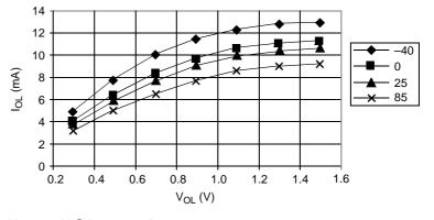
$V_{OL} < 0.3 V @ I_{OL} = 0.5 \text{ mA}$  $V_{OL} < 1.0 V @ I_{OL} = 6.0 \text{ mA}$
