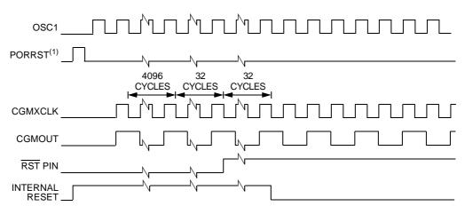
1. PORRST is an internally generated power-on reset pulse.
