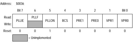
Figure 7-4. PLL Control Register (PCTL)
