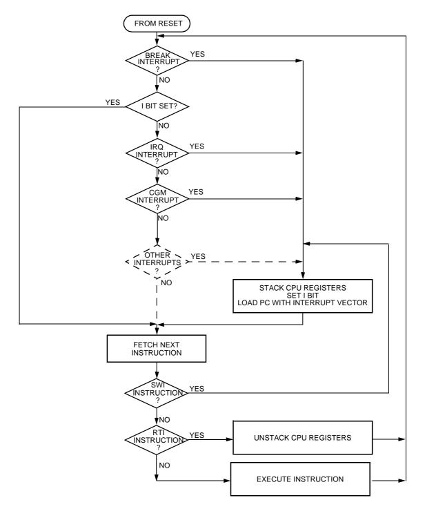
Figure 4-6. Interrupt Processing
