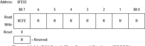
Figure 19-22. SIM Break Flag Control Register (SBFCR)
