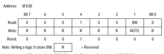
Figure 6-6. SIM Break Status Register (SBSR)
