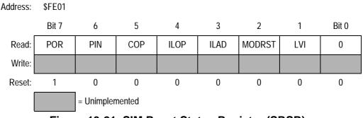
Figure 19-21. SIM Reset Status Register (SRSR)
