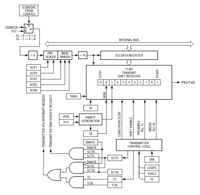
Figure 18-4. SCI Transmitter
