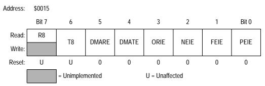
Figure 18-11. SCI Control Register 3 (SCC3)
