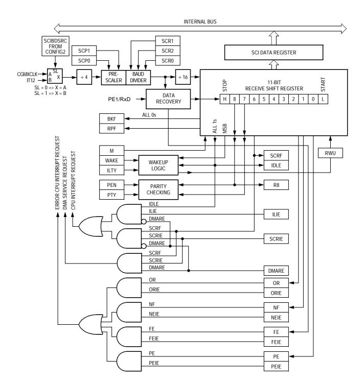
Figure 18-5. SCI Receiver Block Diagram
