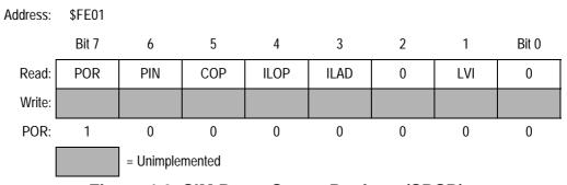
Figure 4-3. SIM Reset Status Register (SRSR)
