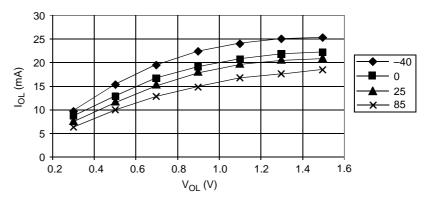
$V_{OL} < 0.8 \ V @ I_{OL} = 10 \ mA$
