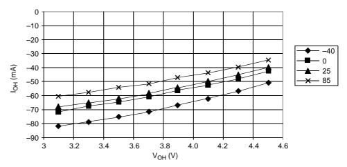
$V_{OH} > V_{DD} - 0.8 \text{ V } @ I_{OH} = -2.0 \text{ mA}$  $V_{OH} > V_{DD} - 1.5 \text{ V } @ I_{OH} = -10.0 \text{ mA}$
