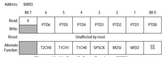
Figure 16-13. Port D Data Register (PTD)
