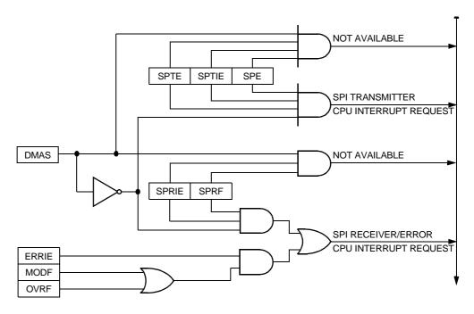
Figure 20-11. SPI Interrupt Request Generation
