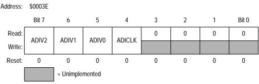
Figure 5-4. ADC Clock Register (ADCLK)
