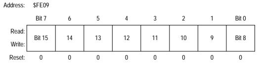
Figure 6-4. Break Address Register High (BRKH)
