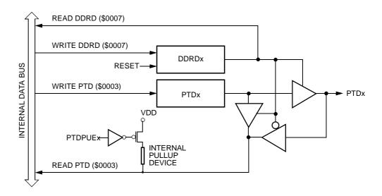
Figure 16-15. Port D I/O Circuit
