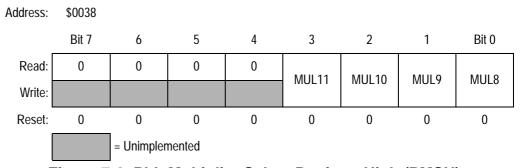
Figure 7-6. PLL Multiplier Select Register High (PMSH)
