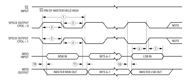
Note: This last clock edge is generated internally, but is not seen at the SPSCK pin.
