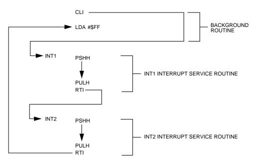
Figure 4-5. Interrupt Recognition Example
