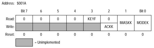
Figure 13-3. Keyboard Status and Control Register (INTKBSCR)
