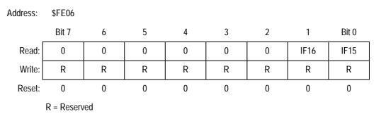
Figure 4-9. Interrupt Status Register 3 (INT3)
