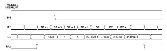
Figure 19-9. Interrupt Recovery Timing
