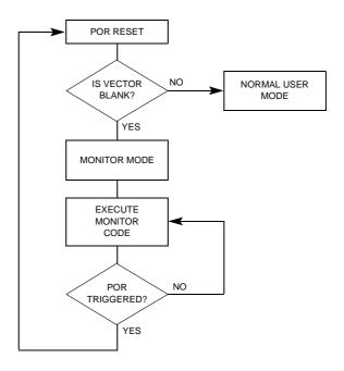
Figure 15-2. Low-Voltage Monitor Mode Entry Flowchart
