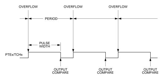
Figure 22-3. PWM Period and Pulse Width
