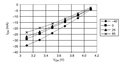
$V_{OH} > V_{DD} - 0.8 \ V @ I_{OH} = -2.0 \ mA$  $V_{OH} > V_{DD} - 1.5 \ V @ I_{OH} = -10.0 \ mA$
