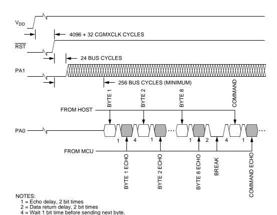
Figure 15-8. Monitor Mode Entry Timing
