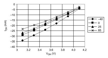
$V_{OH} > V_{DD} - 0.8 \text{ V } @ I_{OH} = -10.0 \text{ mA}$
