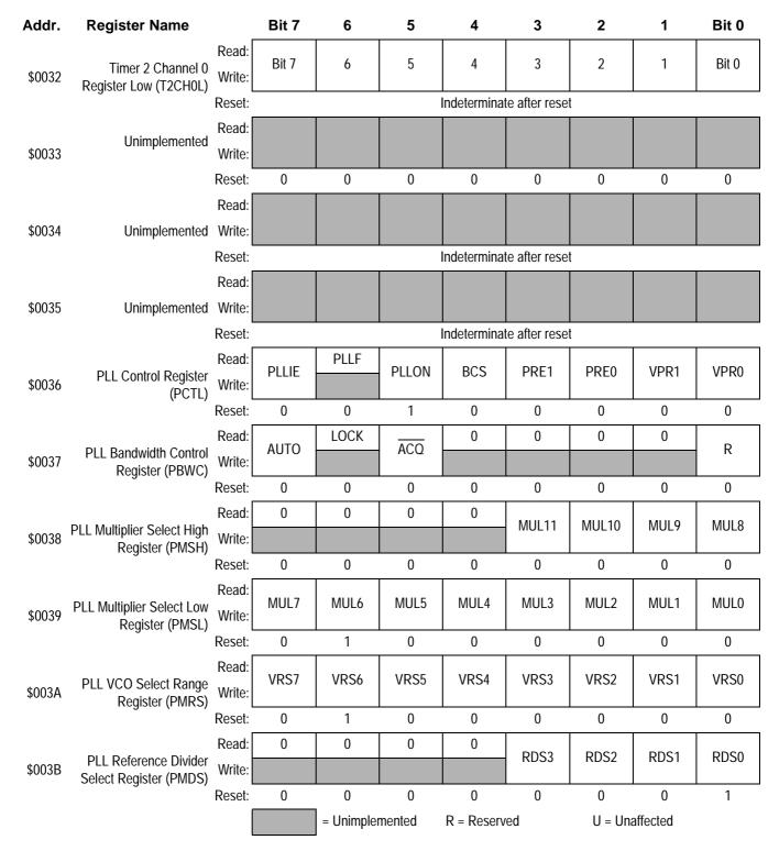
Figure 2-2. Control, Status, and Data Registers (Sheet 6 of 8)
