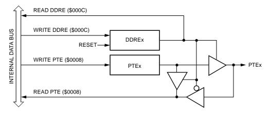
Figure 16-19. Port E I/O Circuit
