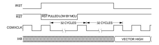
Figure 19-5. Internal Reset Timing
