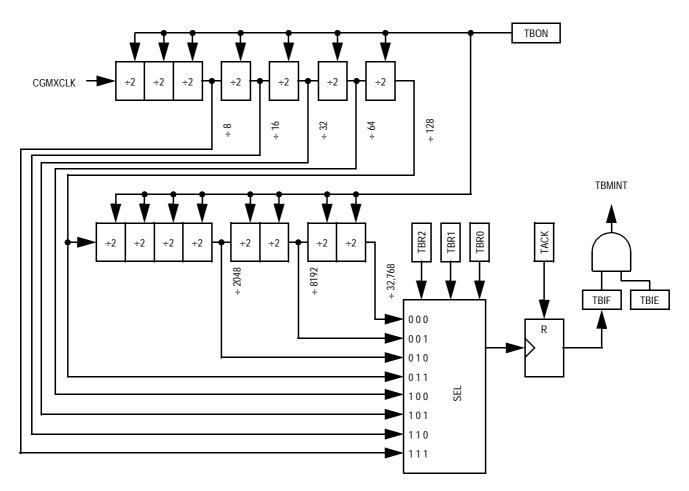
Figure 21-1. Timebase Block Diagram
