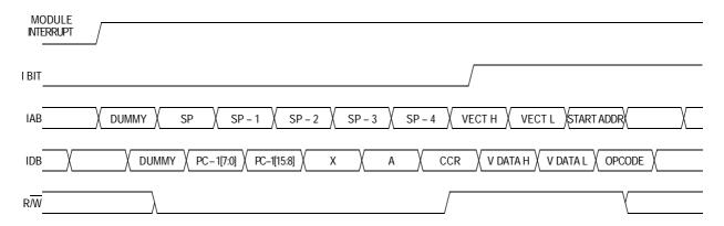
Figure 19-8. Interrupt Entry Timing
