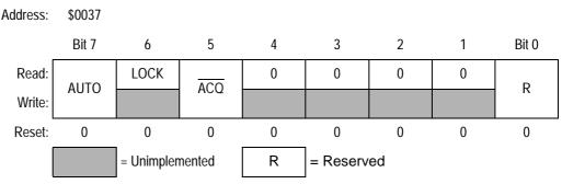
Figure 7-5. PLL Bandwidth Control Register (PBWC)
