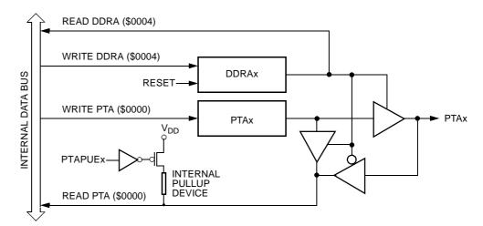
Figure 16-4. Port A I/O Circuit
