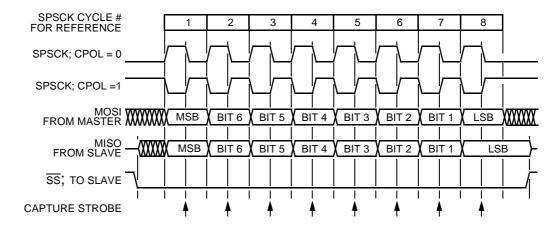
Figure 20-6. Transmission Format (CPHA = 1)
