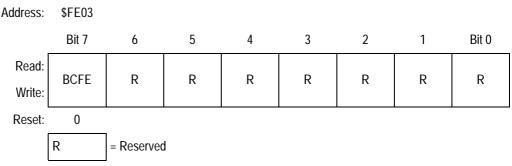
Figure 6-7. SIM Break Flag Control Register (SBFCR)
