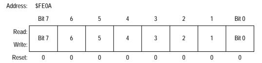
Figure 6-5. Break Address Register Low (BRKL)
