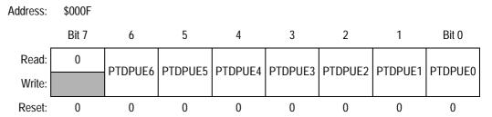
Figure 16-16. Port D Input Pullup Enable Register (PTDPUE)
