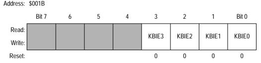
Figure 13-4. Keyboard Interrupt Enable Register (INTKBIER)
