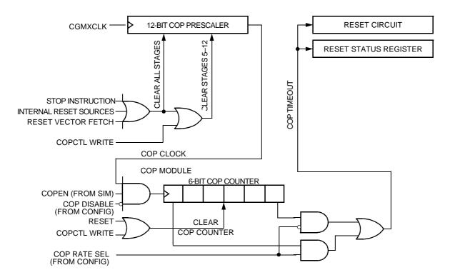
Figure 9-1. COP Block Diagram
