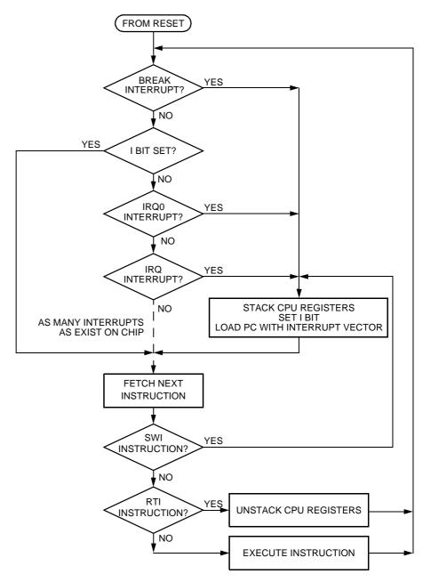
Figure 19-10. Interrupt Processing
