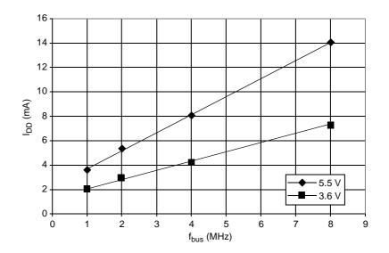
Figure 23-13. Typical Operating  $I_{DD}$ , with All Modules Turned On (–40 °C to 125 °C)
