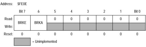
Figure 6-3. Break Status and Control Register (BRKSCR)
