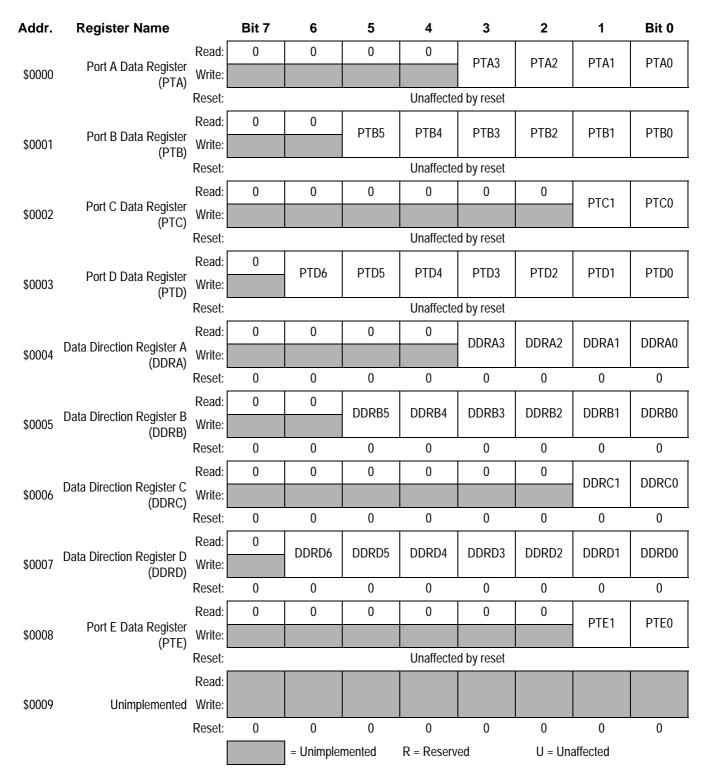
Figure 2-2. Control, Status, and Data Registers (Sheet 1 of 8)
