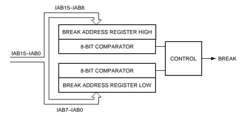
Figure 6-1. Break Module Block Diagram
