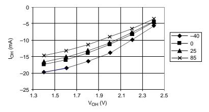
$V_{OH} > V_{DD} -0.3 \text{ V } @ I_{OH} = -0.6 \text{ mA}$  $V_{OH} > V_{DD} -1.0 \text{ V } @ I_{OH} = -4.0 \text{ mA}$
