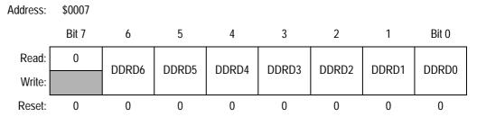
Figure 16-14. Data Direction Register D (DDRD)
