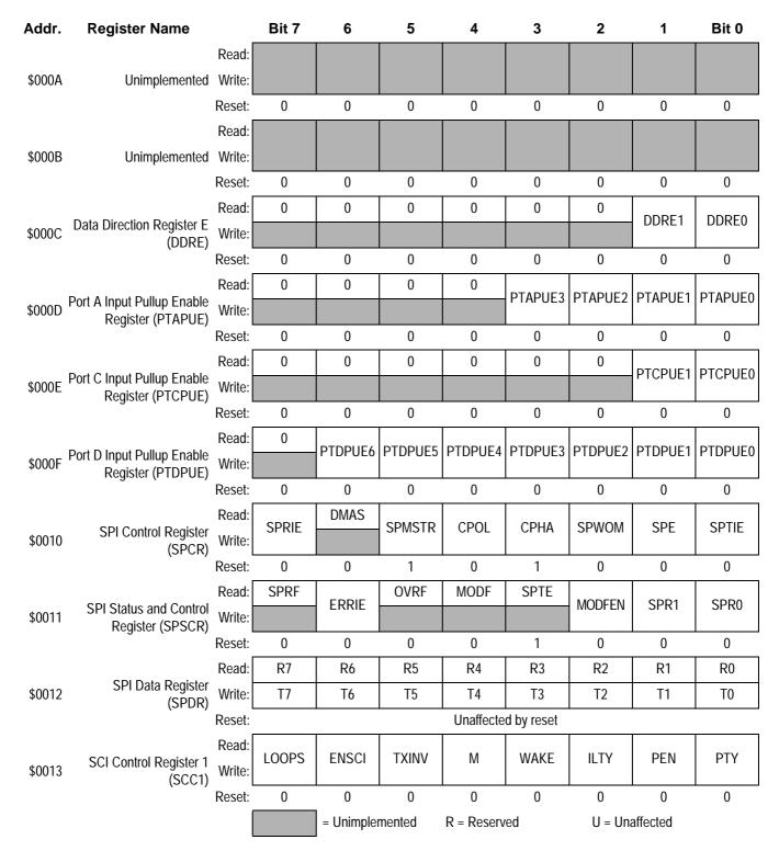
Figure 2-2. Control, Status, and Data Registers (Sheet 2 of 8)
