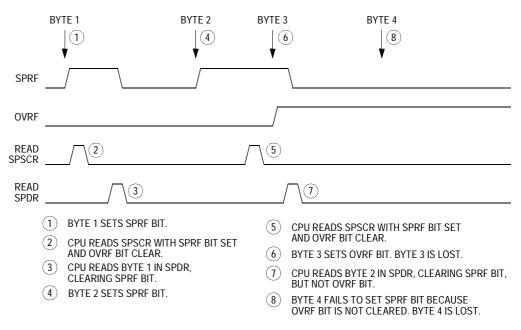
Figure 20-9. Missed Read of Overflow Condition
