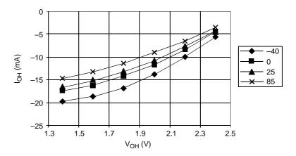
$V_{OH} > V_{DD} -0.3 \text{ V } @ I_{OH} = -0.6 \text{ mA}$  $V_{OH} > V_{DD} -1.0 \text{ V } @ I_{OH} = -4.0 \text{ mA}$
