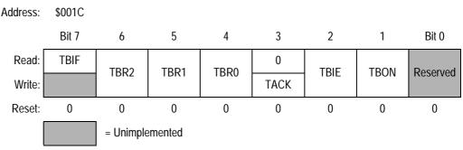
Figure 21-2. Timebase Control Register (TBCR)
