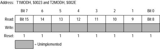
Figure 22-7. TIM Counter Modulo Register High (TMODH)
