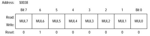
Figure 7-7. PLL Multiplier Select Register Low (PMSL)
