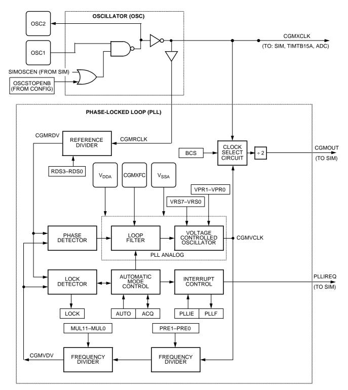
Figure 7-1. CGMC Block Diagram
