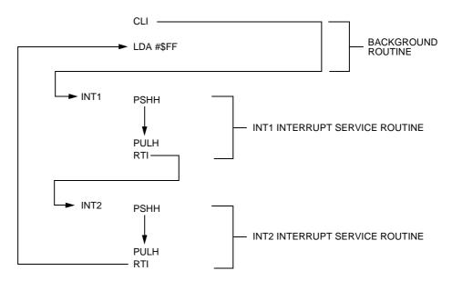
Figure 19-11. Interrupt Recognition Example
