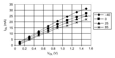
$V_{OL} < 0.4 \ V @ I_{OL} = 1.6 \ mA$  $V_{OL} < 1.5 \ V @ I_{OL} = 10.0 \ mA$
