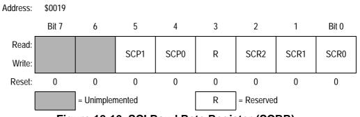
Figure 18-16. SCI Baud Rate Register (SCBR)
