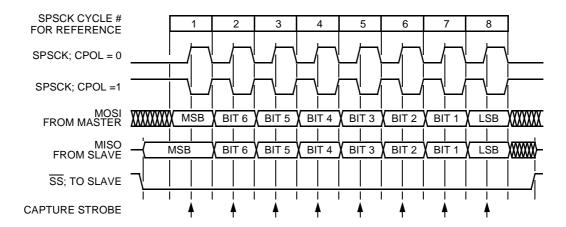
Figure 20-4. Transmission Format (CPHA = 0)
