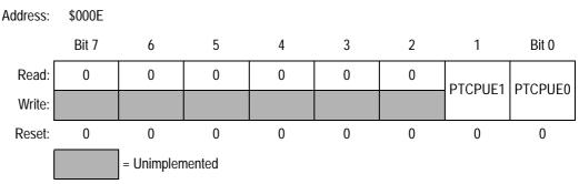
Figure 16-12. Port C Input Pullup Enable Register (PTCPUE)
