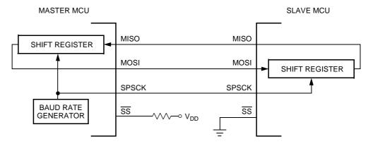
Figure 20-3. Full-Duplex Master-Slave Connections
