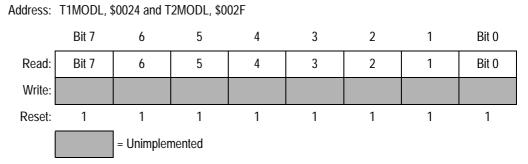
Figure 22-8. TIM Counter Modulo Register Low (TMODL)
