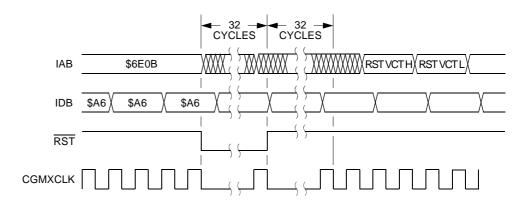
Figure 19-17. Wait Recovery from Internal Reset
