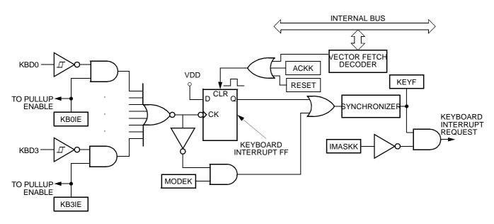
Figure 13-1. Keyboard Module Block Diagram
