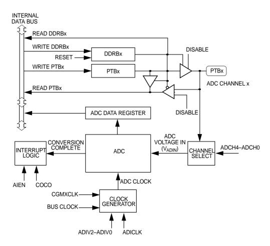
Figure 5-1. ADC Block Diagram
