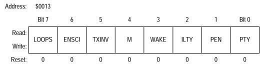
Figure 18-9. SCI Control Register 1 (SCC1)
