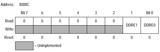
Figure 16-18. Data Direction Register E (DDRE)
