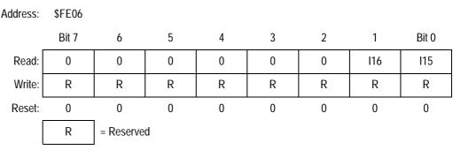
Figure 19-14. Interrupt Status Register 3 (INT3)
