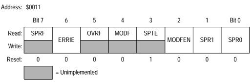
Figure 20-14. SPI Status and Control Register (SPSCR)
