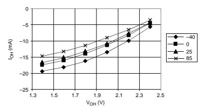
$V_{OH} > V_{DD} - 0.5 \text{ V} @ I_{OH} = -4.0 \text{ mA}$
