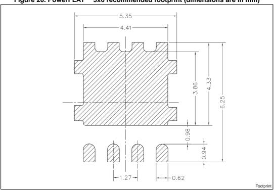
Figure 20. PowerFLAT<sup>™</sup> 5x6 recommended footprint (dimensions are in mm)
