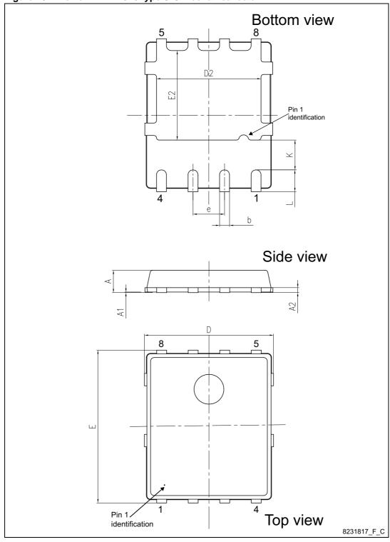
Figure 19. PowerFLAT<sup>™</sup> 5x6 type S-C mechanical data
