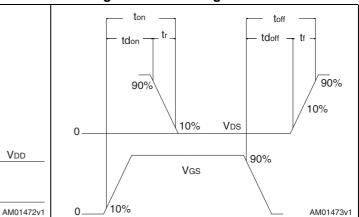
Figure 18. Switching time waveform
