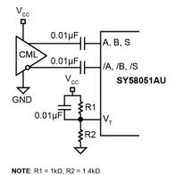
Figure 9. CML Interface (AC-Coupled)
