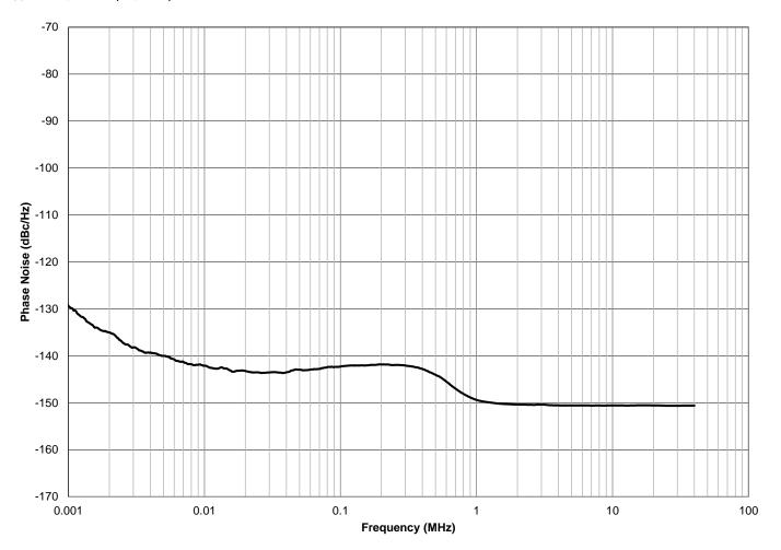
Phase Noise at 622MHz over 12kHz to 20MHz Additive RMS Phase Jitter: 46fs<sub>RMS</sub>
