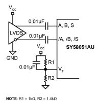
Figure 7. LVDS Interface (AC-Coupled) Note: Be certain that the LVDS driver can be AC-coupled.
