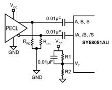
$\begin{array}{l} \textbf{NOTE}\text{: FOR 2.5V, R}_{PD}=50\Omega\text{, R1}=1k\Omega\text{, R2}=1.4k\Omega\\ \text{FOR 3.3V, R}_{PD}=100\Omega\text{, R1}=1k\Omega\text{, R2}=1.4k\Omega \end{array}$
