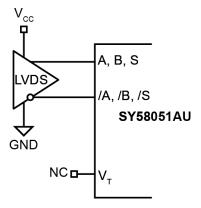
Figure 6. LVDS Interface (DC-Coupled)
