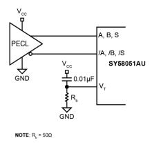
Figure 10. PECL Interface (DC-Coupled)
