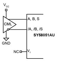
Figure 8. CML Interface (DC-Coupled)
