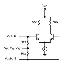
Figure 1. Simplified Differential Input Stage
