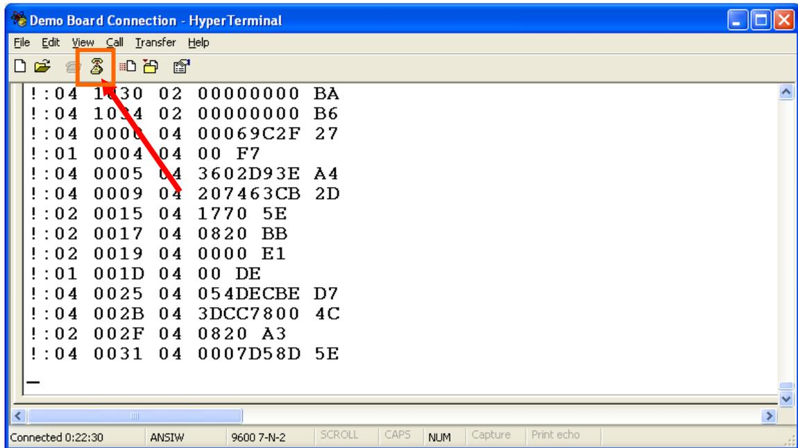
Figure 1-5: Hyperterminal Sample Window with Disconnect Button
