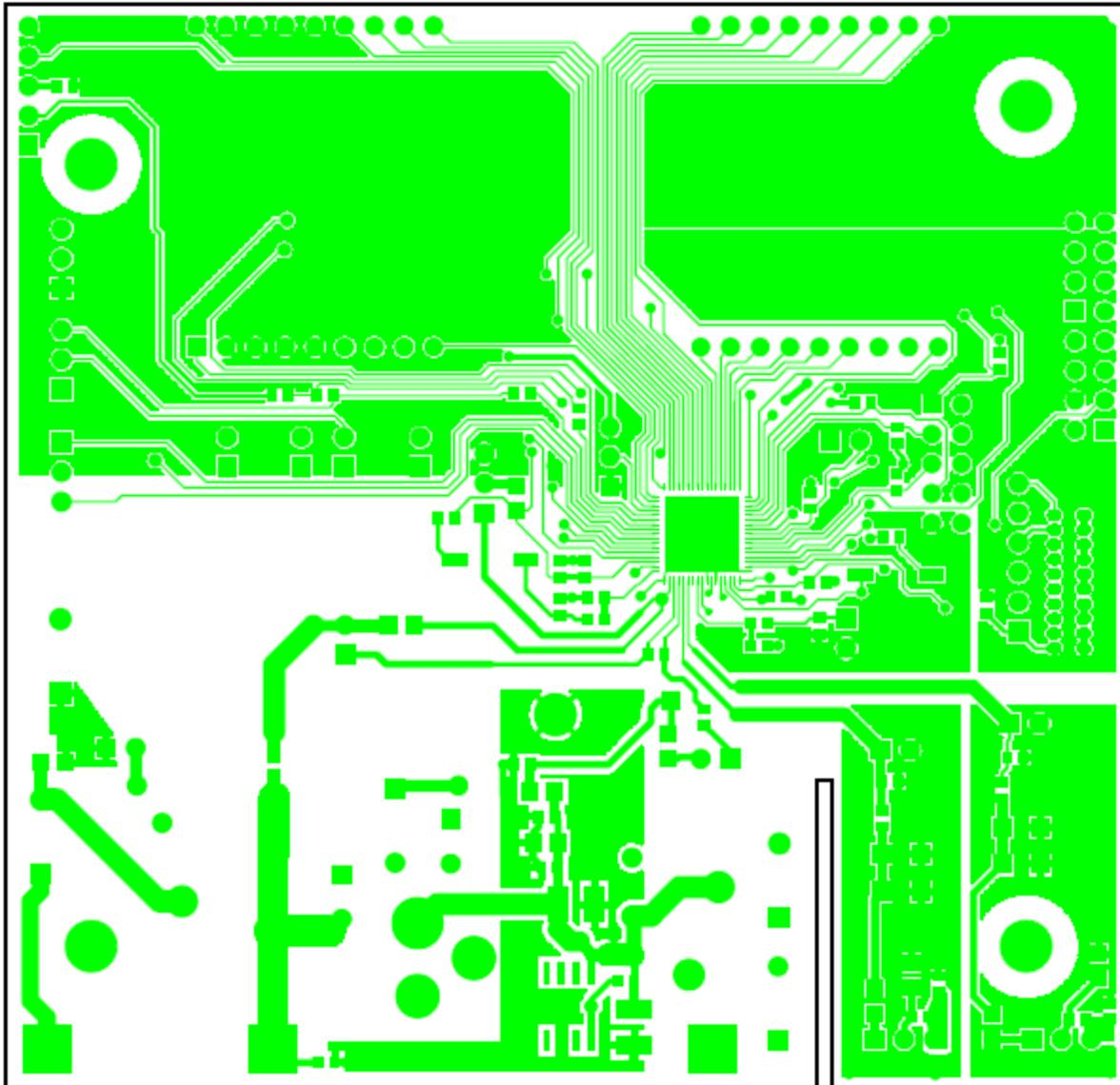
Figure 4-5: 71M6531N12A2 Demo Board: Top Copper Layer
