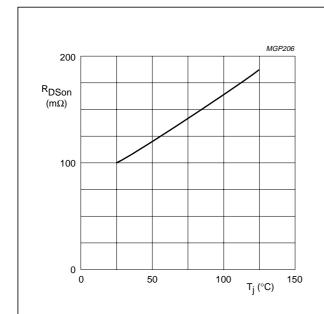
Drain-source on-state resistance as a function of junction temperature; typical values per section.
