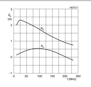
Class-AB operation;  $V_{DS} = 28 \text{ V}$ ;  $I_D = 2 \times 250 \text{ mA}$ ;
