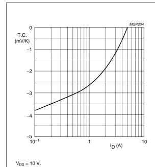
Temperature coefficient of gate-source Fig.4 voltage as a function of drain current; typical values per section.
