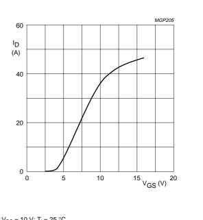
$V_{DS} = 10 \text{ V}; T_j = 25 ^{\circ}\text{C}.$
