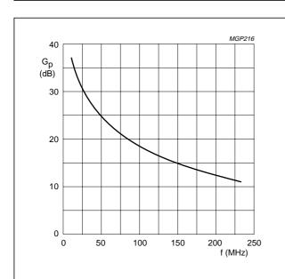
Class-AB operation;  $V_{DS} = 28 \text{ V}$ ;  $I_D = 2 \times 250 \text{ mA}$ ;
