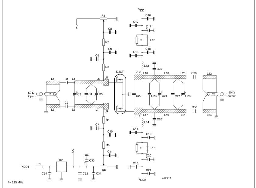
Fig.11 Test circuit for class-AB operation.
