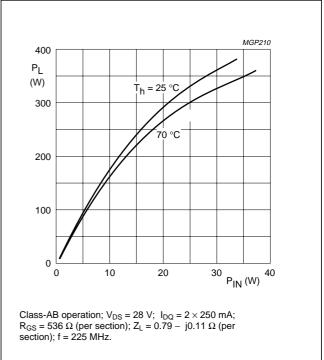
Fig.10 Load power as a function of input power; typical values.
