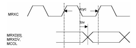
Figure 10. SNI (7-wire) Output Timing
