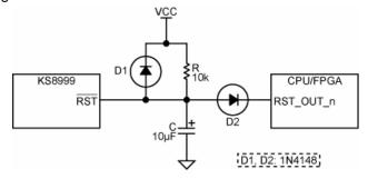
Figure 20. Recommended Reset Circuit
