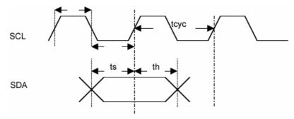
Figure 7. EEPROM Input Timing
