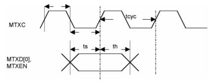
Figure 9. SNI (7-wire) Input Timing
