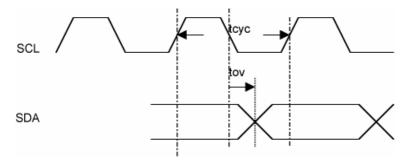
Figure 8. EEPROM Output Timing
