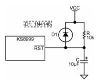
Figure 21. Recommended Circuit for Interfacing with CPU/FPGA Reset
