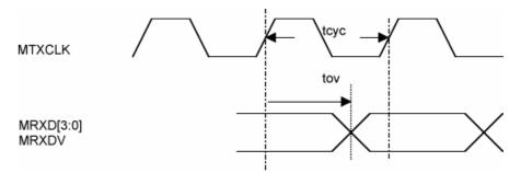
Figure 14 KS8999 PHY Mode Transmit Timing
