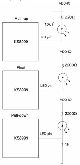
Reference circuits for unmanaged programming through LED ports Note: For brighter LED operation use VDD-IO = 3.3V
