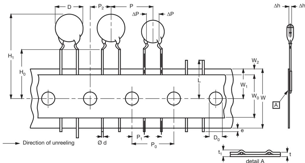
Kinked capacitors on tape, lead spacing 5.0 mm (0.2")
