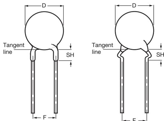
Capacitors with 7.5 mm (0.30") and 10 mm (0.40") lead spacing
