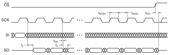
Figure 13-3. HOLD Timing – Serial Input
