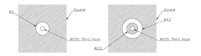
\*The antenna feeding in transmission line should connect with the  $\varphi$  2.5 circle at the Bottom Side, and keep transmission line impedance at 50 ohms for good power transmit from system to antenna.
